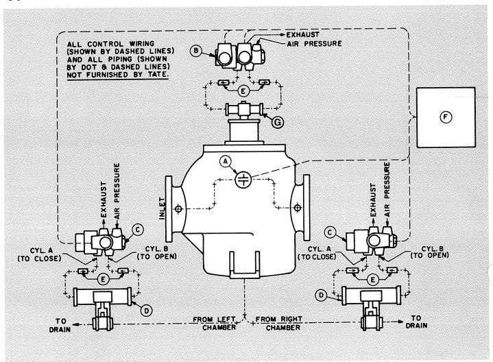
This is a completely automatic system with air-operated flushing valve controlled by an impulse from a differential pressure switch connected across the inlet and outlet nozzles of the strainer.
