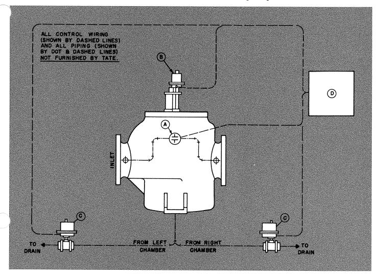
This is a completely automatic system with electrical flushing valves controlled by an impulse from a differential pressure switch connected across the inlet and outlet nozzles of the strainer.
