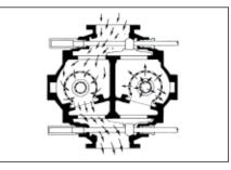
Water for the spray pipes can be taken from the strainer discharge provided the pressure is 50 PSIG or higher, or from a separate source. There must be no back pressure on the drain line, and the line must be large enough to keep the compartment drained. These strainers are suitable for vacuum or positive pressure operation.
